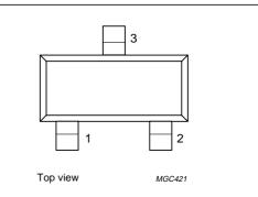
Fig.1 Simplified outline (SOT23) and pin configuration.
